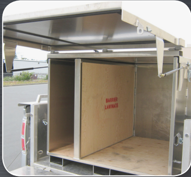
SEPARATED STORAGE FOR POWDER AND DETONATORS
